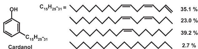
Figure 1. Chemical structure of cardanol used in this study.
